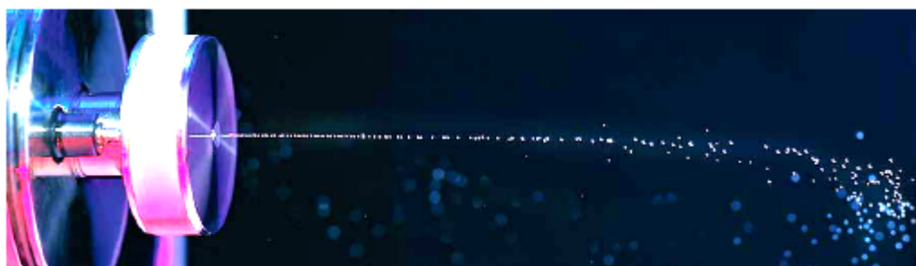
Figure 5-31: Picture of operating vibrating orifice from VOAG datasheet (TSI Model 3450 VOAG datasheet). ‘Haze’ around particle stream could be sub-micron particles.
